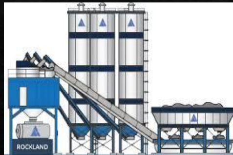
Concrete Batch Plant
